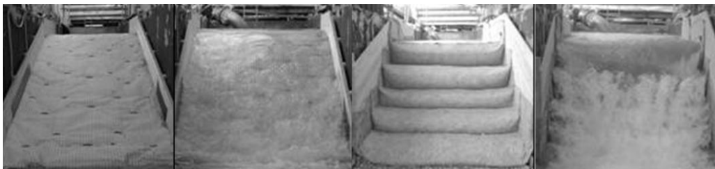
Fig. 5. Loaded and unloaded dike models with slope parallel geosynthetic layers using anchors for fixation (left) and wrap-around method (loops) (right) (Haselsteiner et al., 2008)
