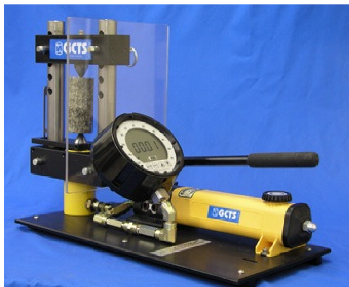
Figure 1. Picture of a point load test rig device (Avantech Engineering Consortium Pvt, 2015)
