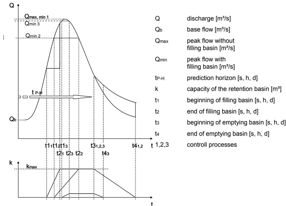
Figure 4: Control process and utilization of the capacity  $k$  based on Fischer (2007)
