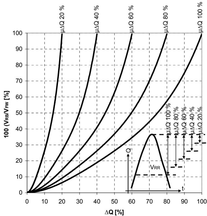
Figure 7: Actual flood peak reduction depending on the utilization of the theoretical flood peak reduction
