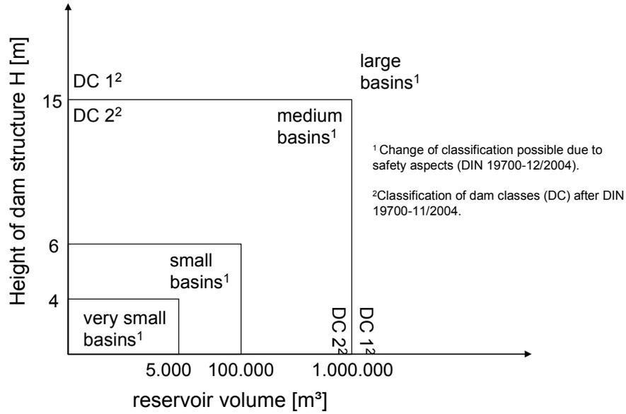
Figure 2: Classification of flood retention basins according to DIN 19700-12/2004
