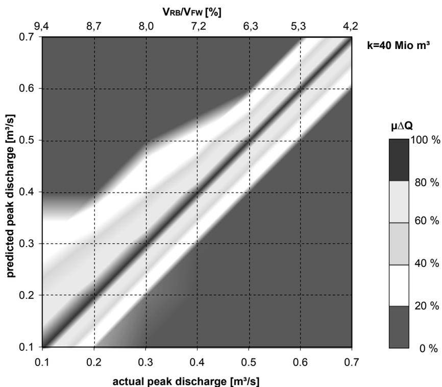
Figure 6: Utilization levels of the theoretical flood peak reduction
