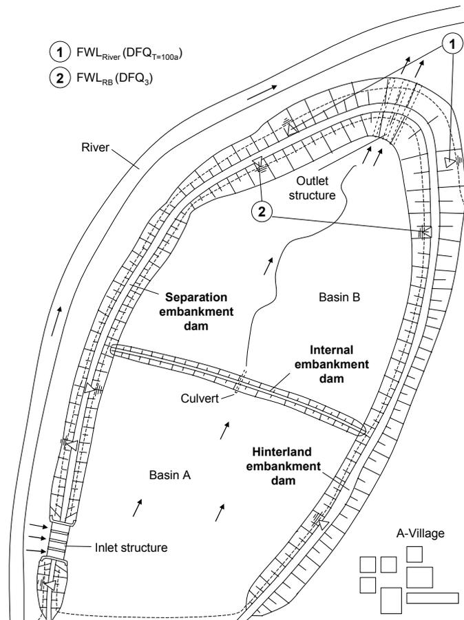
Figure 1: Typical bypass flood-control retention basin along rivers based on Haselsteiner (2007a)
