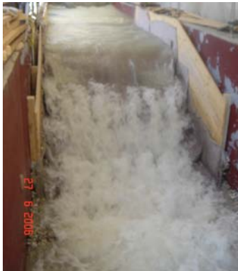
Figure 7. Method (III) – Overflow with integrated defense design using geocomposite envelopes, slope 1:n = 1:1.5, q = 130 \text{ l/(s-m)} (Haselsteiner 2008)
