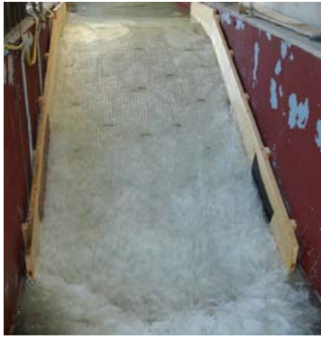
Figure 6. Method (II) – Overflow with embankment stabilization system using geogrids and geocomposites (nails up), slope 1:n = 1:2.5, q = 300 \text{ l/(s-m)} (Haselsteiner 2008)
